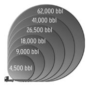
Select Tanks are available in a variety of sizes ranging from 4,500 to 62,000 barrels. Our largest tank replaces over 120 standard frac tanks, reducing costs associated with transport, set up and removal.
