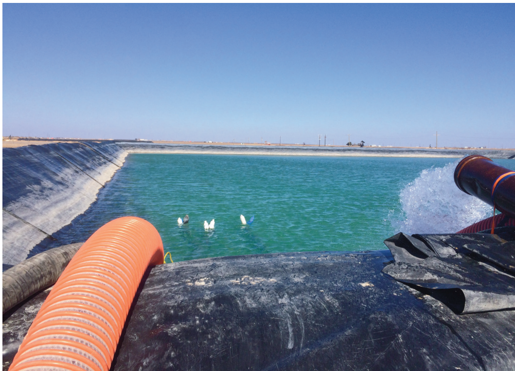
Figure 3. Fresh water pit, used by Select to draw from and blend with recycled water on the frack pad for controlled blend ratios via an automated mixing manifold with concentration sensors.
